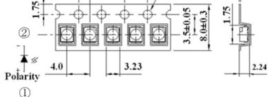
Note: Tolerances unless mentioned ±0.1mm. Unit = mm
