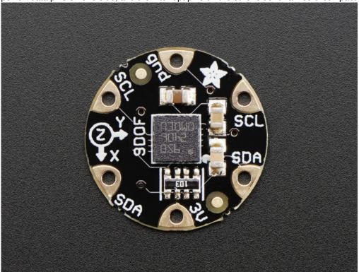
The **Flora** version has just I2C interface for a super-small design. Attaching it to the FLORA is simple: line up the sensor so its adjacent to the SDA/SCL pins and sew conductive thread from the 3V, SDA, SCL and GND pins. They line up perfectly so you will not have any crossed lines. You can only connect one of these sensors to your FLORA, but you can connect other I2C sensors/outputs by using the set of SCL/SDA pins on the opposite side.
