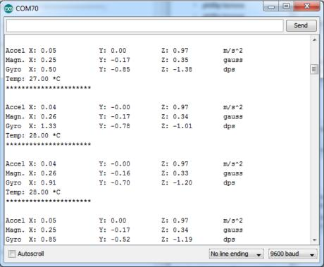
We suggest using this Adafruit\_Sensor interface version, since it will let you swap sensors without having to worry about units compatibility. Try twisting and moving the board around to see the sensors change value.
