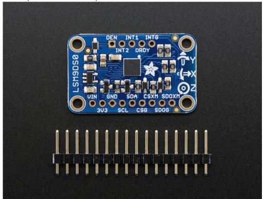
The **breakout board** version of this sensor has both I2C and SPI interfaces. Attaching it to the Arduino is simple, power Vin and GND with 3-5VDC, and wire up I2C data on SCL and SDA, and you're ready to go! More advanced users can use SPI, our library has support for both. The breakout comes fully assembled and tested, with some extra
