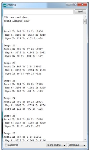
This output is not terribly useful for most people - its simpler but does not have adjusted output units. Instead, we suggest the **sensorapi** demo. Upload that to the Arduino and open up the Serial console again.
