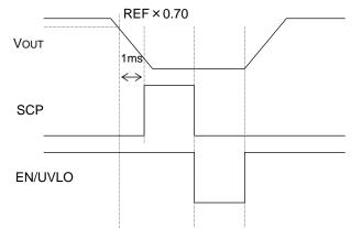
When output voltage (Is-) falls to  $\mathsf{REF} \times 0.7$  or less, SCP comparator inside IC is exercised.
