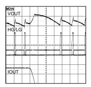
Fig.18 Transient Response (VIN=19V)
