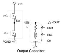
When determining the proper output capacitor, be sure to factor in the equivalent series resistance and equivalent series inductance required to set the output ripple voltage 20mV or more. In selecting the limit of inductor, be sure to allow enough margin for output voltage.
