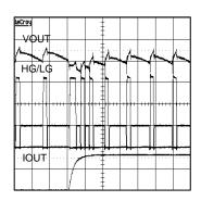
Fig.15 Transient Response (VIN=19V)
