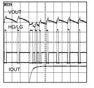
Fig.14 Transient Response (VIN=12V)
