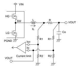
When the output voltage is 2.7V or more, use the resistance for setting output voltage like left figure, for Is+ and Is-.
