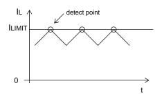
As soon as the voltage drop between Is+ and Is- generated by the inductor current becomes specific threshold, the gate voltage of the high side MOSFET becomes low.
