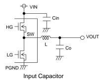
The input capacitor selected must have low enough ESR resistance to fully support large ripple output, in order to prevent extreme over current. The formula for ripple current IRMS is given in (9) below.
