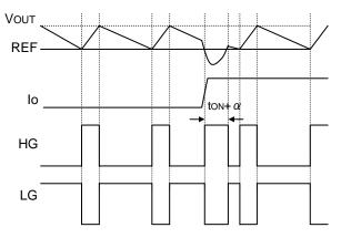
When VOUT drops due to a rapid load change, and the voltage remains below VREF after the programmed ton time interval has elapsed, the system quickly restores VOUT by extending the ton time, improving the transient response.
