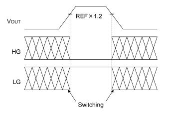
When output rise to or above REF  $\times$  1.2, output over voltage protection is exercised, and low side FET goes up maximum for reducing output. (LG=High, HG=Low). When output falls, it returns to the standard mode.
