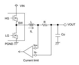
The over current protection function detects the output ripple current peak value. This parameter (setting value) is determined as in formula (10) below.
