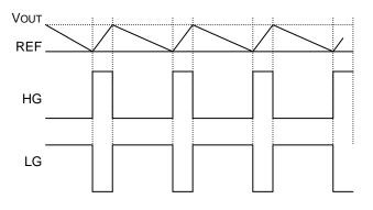
When VOUT falls to a threshold voltage (REF), the drop is detected, activating the  $H^3Reg^{TM}$  CONTROLLA system.
