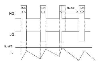
During the normal operation, when VOUT becomes less than REF Voltage, HG becomes High during the time ton (P9). However, when inductor current exceeds  $I_{\text{LIMIT}}$  threshold, HG becomes OFF.
