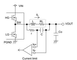
When the over current protection is detected by DCR of coil L, this parameter (setting value) is determined as in formula (11) below.
