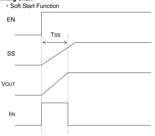
Soft start is exercised with the EN pin set high. Current control takes effect at startup, enabling a moderate output voltage "ramping start." Soft start timing and incoming current are calculated with formulas (2) and (3) below.
