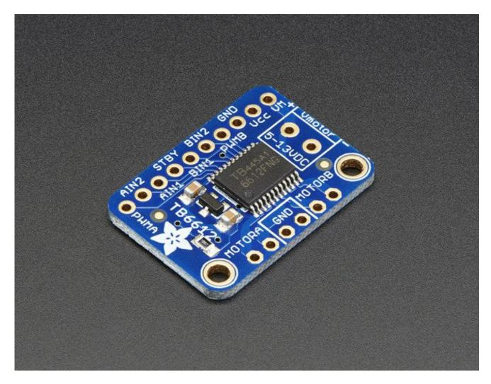
Fire four solenoids, spin two DC motors or step one bi-polar or uni-polar stepper with 1.2A per channel using the TB6612. These are perhaps better known as "the drivers in our assembled Adafruit Motorshield (http://adafru.it/1438) or Motor HAT (http://adafru.it/eRq)" We really like these dual H-bridges, so if you want to control motors without a shield or HAT these are easy to include on any solderless breadboard or perma-proto.
