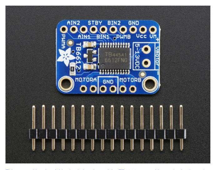
This motor driver is a fairly simple breakout of the TB6612 motor chip, so do check out the datasheet for the TB6612 for any details you need about pin voltage limits, capacitance, etc! (http://adafru.it/emK)
