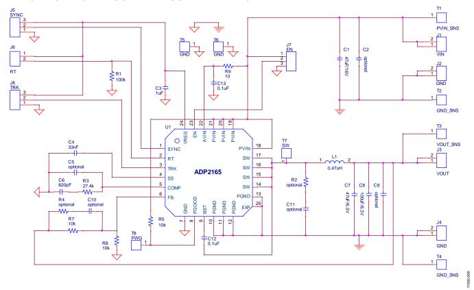
Figure 4. Schematic of the ADP2165-EVALZ
