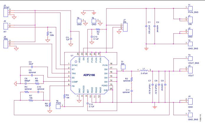
Figure 5. Schematic of the ADP2166-EVALZ
