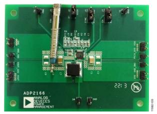
Figure 3. Output Ripple Measurement
