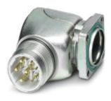
Device connector, front mounting, angled rotatable, Screw locking, M23, Number of positions: 4+3+PE, Type of contact: Pin, Crimp connection, Axial O-ring, 4x Ø 3.2, shielded: yes, Flange dimensions: 28 mm x 28 mm, Compatible with mating connectors with SPEEDCON or M23 standard knurled nuts
