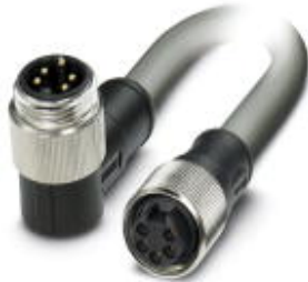
Bus system cable, DeviceNet, 5-position, PVC, Gray RAL 7001, Plug angled 7/8"-16UNF, on Socket straight 7/8"-16UNF, Cable length: 5 m
