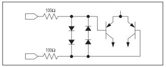
Figure 2. Input Protection Circuit
