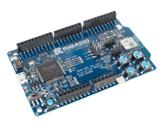
It is designed for ease of use while still providing full access to the features of the BMD-340. The built-in USB programmer allows for easy programming and configuration. All the I/O are accessible and Arduino R3 form factor connectors support plug-and-play accessory shields.
