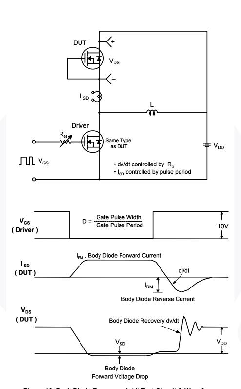
Figure 16. Peak Diode Recovery dv/dt Test Circuit & Waveforms
