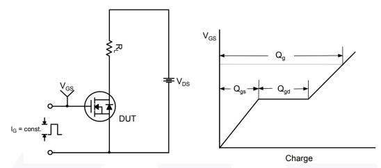
Figure 13. Gate Charge Test Circuit & Waveform
