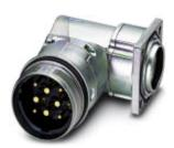
Device connector, front mounting, angled rotatable, SPEEDCON locking, M40, Number of positions: 4+3+PE, Type of contact: Male connector, Crimp connection, Axial O-ring, 4xØ4,4, Shielded: Yes, Flange dimensions: 40 mm x 40 mm
