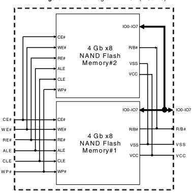
Figure 4.2 Block Diagram — 1 CE (4 Gb x 8)
